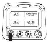
2. The main menu will pop up on the display. Use the "Arrow Buttons" to scroll through the menu until the "Setup 1-up Display" is highlighted.
